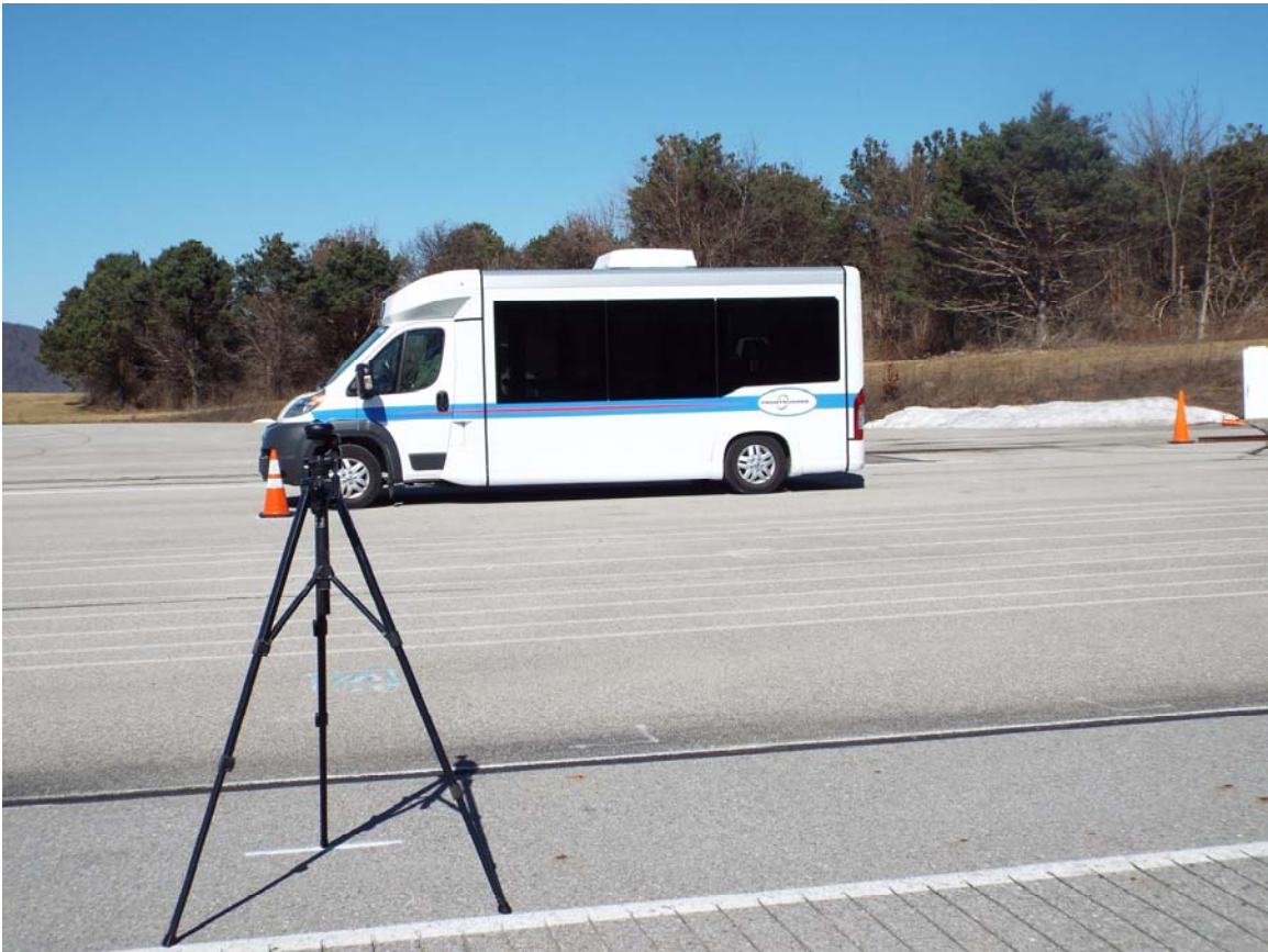
TEST BUS UNDERGOING EXTERIOR NOISE TESTING
