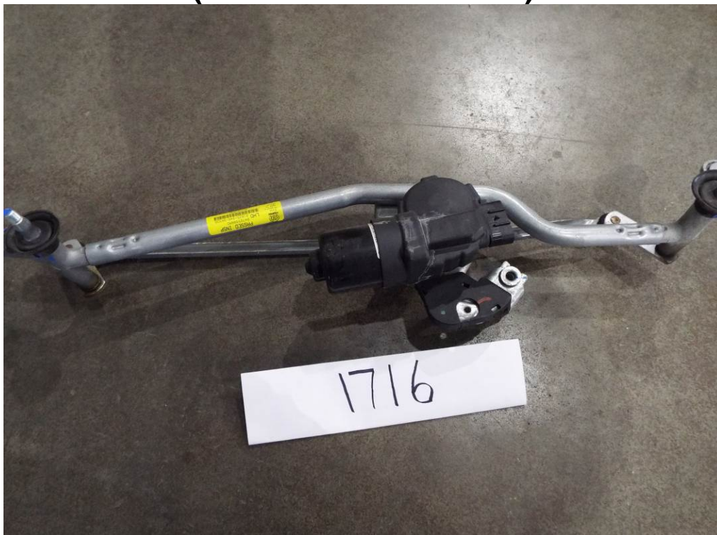
WIPER MOTOR REMOVAL AND REPLACEMENT (0.75 LABOR HOURS)
