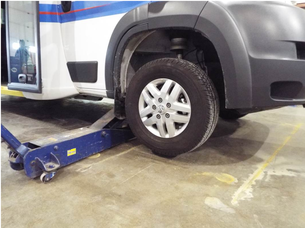
PLACEMENT OF JACK- FRONT AXLE
