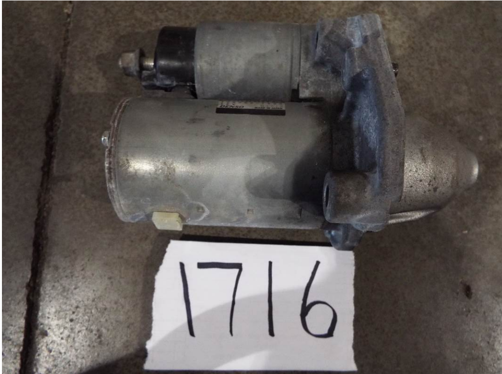
STARTER REMOVAL AND REPLACEMENT (1.50 LABOR HOURS)
