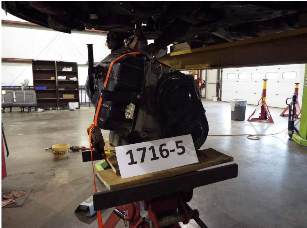
TRANSMISSION REMOVAL AND REPLACEMENT (8.50 LABOR HOURS)
